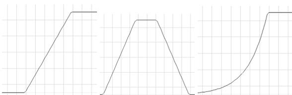
**Figure 4:** The linear, delta, and exscale parametric profile function shapes.
