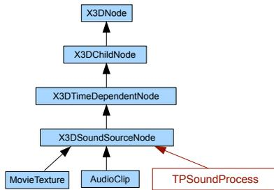
**Figure 1:** The proposed element `TPSoundProcess` extending `X3DSoundSourceNode`.
